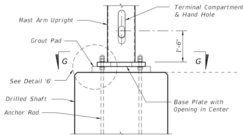
**BASE PLATE & ANCHORAGE ELEVATION**
