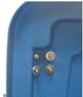
1. Pre-drill 3/16" holes for the hasp hinge in the two top, front corners (A) of the body of the can.
