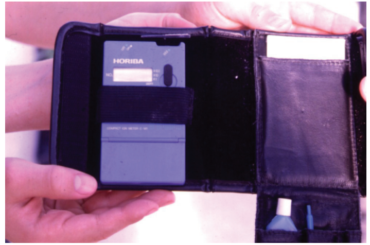
Figure 7. Ion-specific meters for measuring petiole sap nitrate and potassium concentrations.
