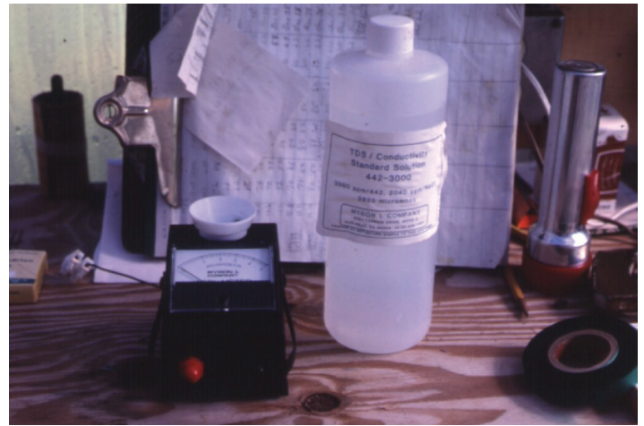
Figure 6. Conductivity meter and standard solution for routine calibration of meter.
