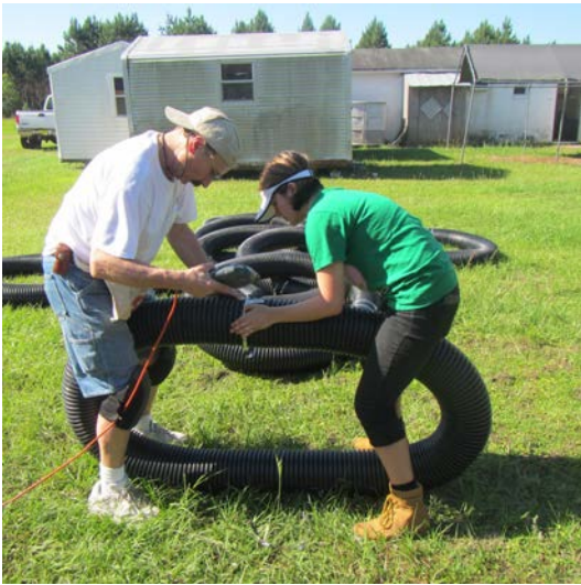
Figure 2A. Large corrugated tubing was used to create floating rings. The tubing was attached to cylinders of plastic (Aquatic Research Instruments, Hope ID) to create the mesocosm area.
