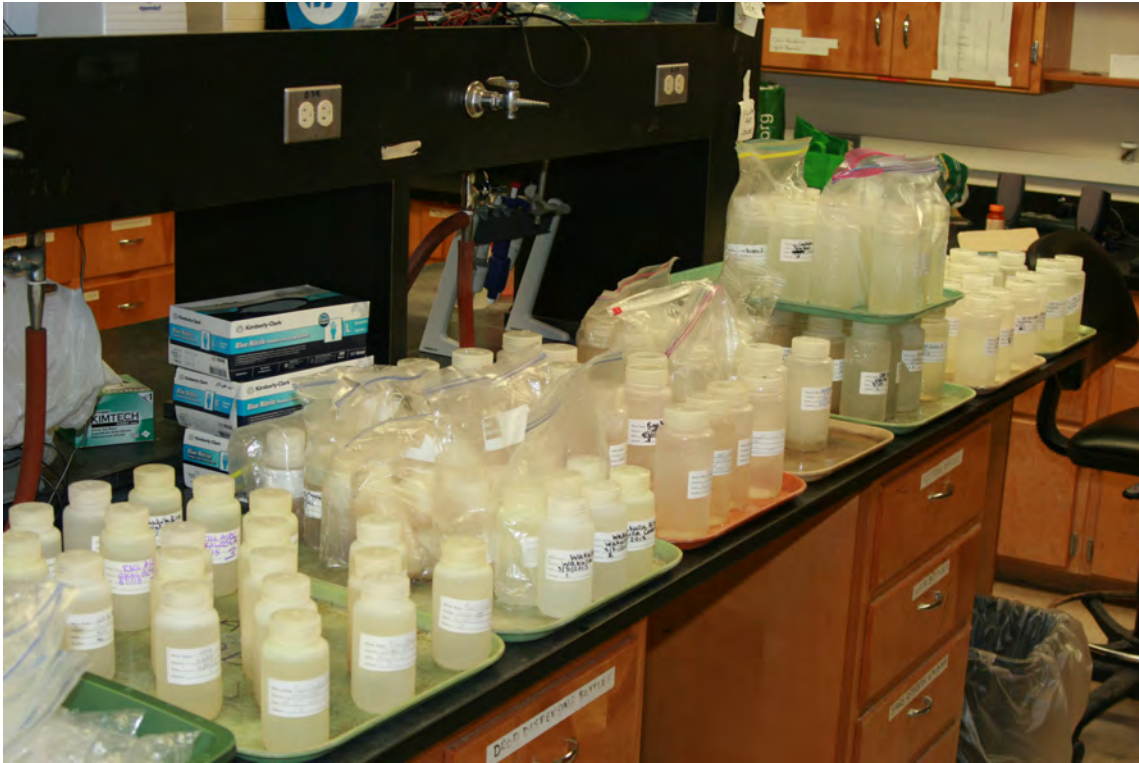
Sample bottles ready for total phosphorus and total nitrogen analysis.
