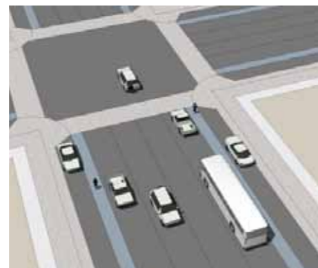
Good: Lanes, No Median, Bike Lanes, Sidewalks.
