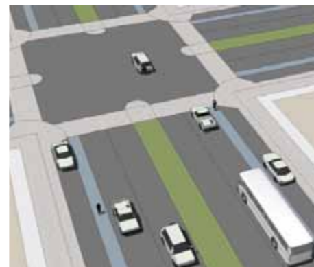
Best: Lanes, Bike lanes, Median, Sidewalks.
