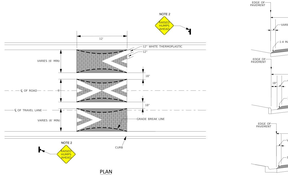
4. SPEED CUSHION SHALL BE 20' MINIMUM FROM DRIVEWAY FLARE, 50' FROM INTERSECTION P.C., AND 100' MINIMUM FROM ANY STOP OR SIGNAL CONTROLLED INTERSECTIONS.
